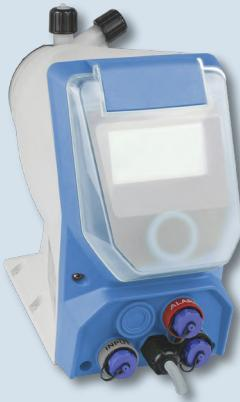
Stepper motor-driven diaphragm dosing pump for ultra-precise dosing of liquid media. The turndown ratio of 1:4800 ensures precise and uniform dosing. The slow-motion mode enables dosing of higher viscosity media up to 10,000 CPS.
