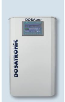
Compact chlorine dioxide unit operating according to the unpressurised chlorite/acid pro-cess.  ${\rm ClO}_2$  output: 0 – 5, max. 30 g/h (depending on the system capacity). Can easily be expanded for a multiple disinfection system.
