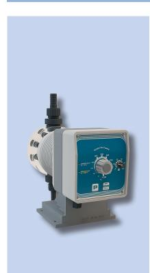
Solenoid-driven diaphragm dosing pump for high viscosity media up to 50,000 cPs for the capacity range between 0-40 l/h.
