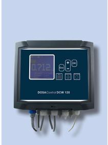
Single channel controller, freely programmable for the following potentiostatic sensors: pH, redox (ORP), conductivity, temperature, turbidity, oxygen, nitrate. For amperometric sensors: Cl<sub>2</sub>, COl<sub>2</sub>, O<sub>3</sub>, H<sub>2</sub>O<sub>2</sub>, PES, bromine, each for a mA or a mV signal input.
