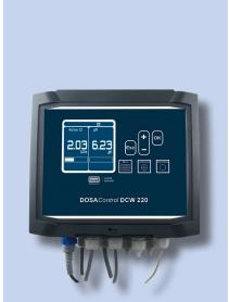
2-channel controller, freely programmable for potentiostatic and amperometric sensors, for measurement of: pH, free chlorine, total chlorine, chlorine dioxide, ozone, oxygen, conductivity, temperature, redox or turbidity.
