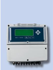
3-channel controller for potentiostatic and amperometric sensors, for measuring and control: pH, redox, free chlorine or total chlorine, chlorine dioxide, bromine, ozone, hydrogen peroxide or peracetic acid and for measuring and indicating temperature.
