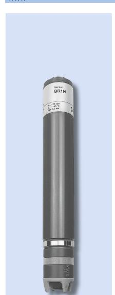
Membrane-covered, amperometric potentiostatic 3-electrode system. Detects free bromine as hypobromous acid and BCDMH, also in sea water.
