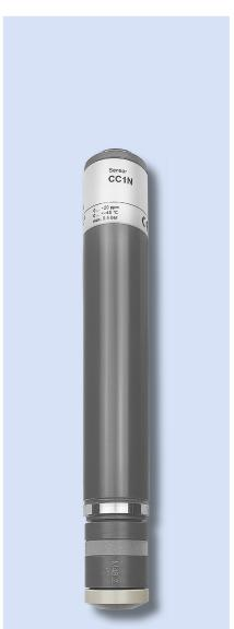
Chlorine sensor with membrane-covered, amperometric 3-electrode system. For the measurement of free chlorine on the basis of iso-cyanuric acid, also in seawater, with reduced pH dependence.
